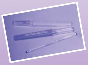
Spirit-filled or digital thermometers are as accurate as mercury thermometers for most applications. Since they are mercury-free, no mercury will be released if they break in the home, laboratory or outdoors, or when they are thrown away. Digital thermometers last longer because they do not break. Consequently, they cost less in the long run.
